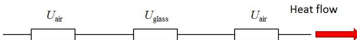
Figure 165 Modelling heat flow through layers of air as well as glass
