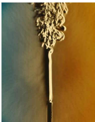
Figure 111 Changing from laminar to turbulent flow
