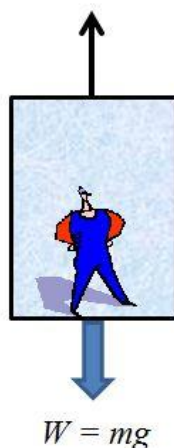
Figure 1 Feeling your normal weight when going up at constant speed.
