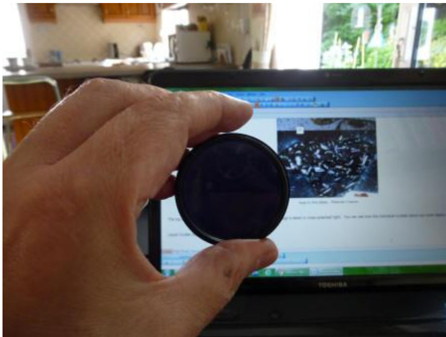
Figure 85 Holding a polarising filter to a computer screen
