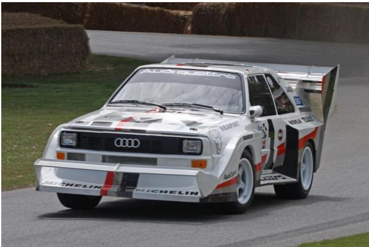
Figure 102 Inverted aerofoil on a racing car (Image by Brian Snelson - Wikimedia Commons)
